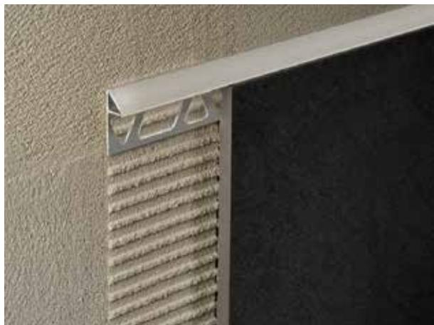
TRIALJOLLY TJ profiles elegantly trim wainscot walls and provide an angled transition to the upper wall surface. The 45° decorative profile aesthetically finishes the otherwise sharp tile edge.
